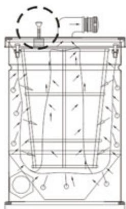
The Manual Filter Shaker system allows the operator to clean the main filter without having to open the vacuum cleaner. This shaker System reduces maintenance down time.
